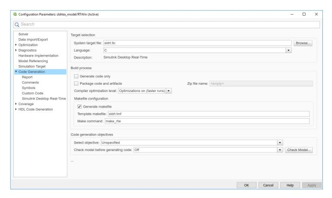
Do not set **Default parameter behavior** to Inlined on the **Optimization** node under **Code Generation**. Inlining parameters is for custom targets when you want to reduce the amount of RAM or ROM with embedded systems. Also, if you select inlining parameters, you disable the parameter tuning feature. Do not inline parameters because PCs have more memory than embedded systems.
